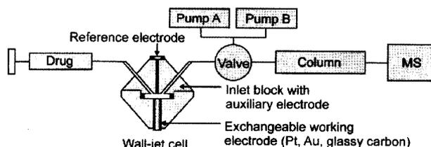
**Fig. 2.** Online EC–LC–MS set-up for the electrochemical generation of oxidative metabolites with subsequent LC separation and detection by mass spectrometry. A 10-port valve equipped with a 10- $\mu$ l injection loop allows the use of low flow rates (10  $\mu$ l/min) for the electrochemical conversion in combination with high flow rates for the LC separation (400  $\mu$ l/min).
